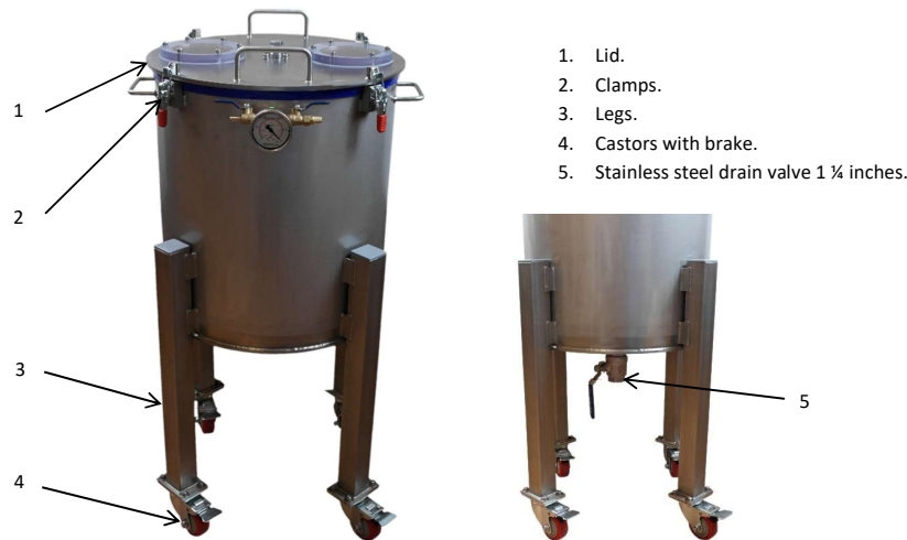
Photo 13: Vacuum chamber with stirrer mechanism.
