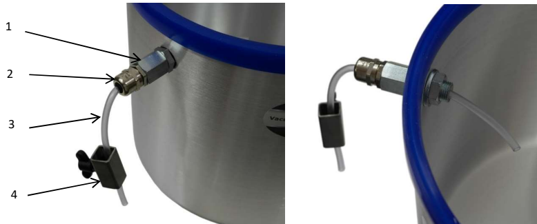
Photo 10: Vacuum feedthrough with pouring hose and flow controller mounted on the tank.
