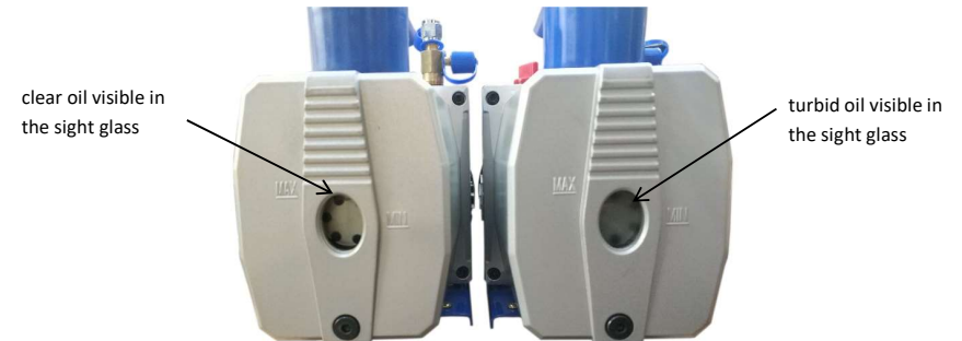
Photo 19: The result of the cold trap work - oil in vacuum pumps clarity (left: clear oil when using a cold trap, right: turbid oil when no cold trap is used).
