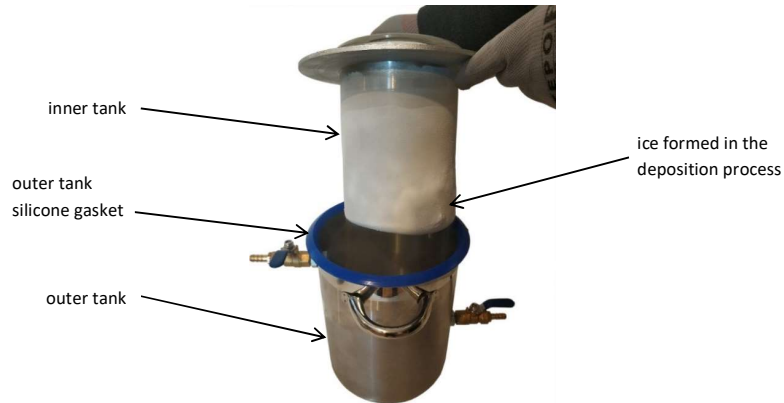
Photo 17: Inner tank, outer tank, silicone gasket and ice formed on the internal tank.
