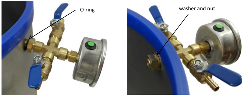
Photo 4: Air manifold inserted into the hole.
