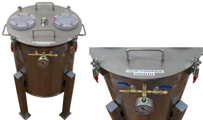
Photo 14: Correct location of the lid on the chamber.
