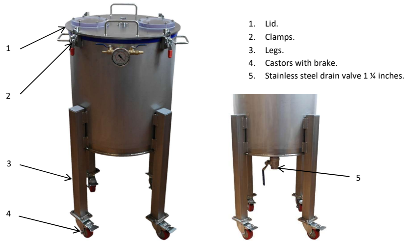
Photo 13: Vacuum chamber with stirrer mechanism.
