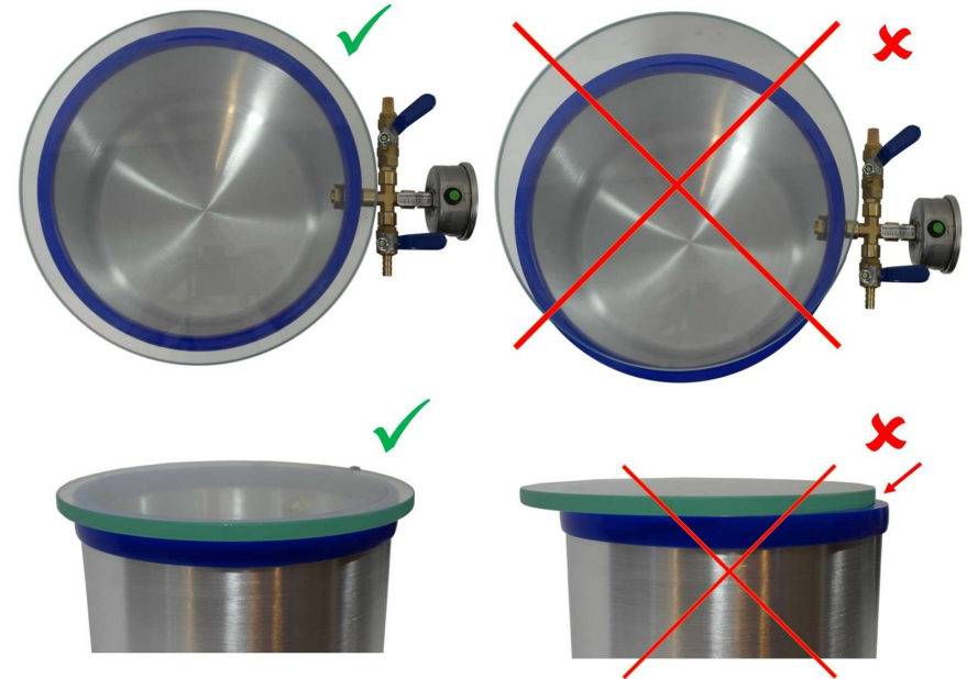
Photo 20: Correct (left) and incorrect (right) positioning of the lid on the chamber.
