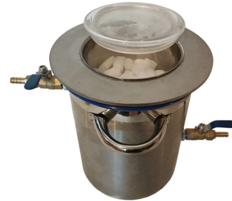
Photo 18: Vacuum cold trap with dry ice inside.
