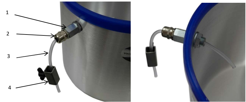
Photo 10: Vacuum feedthrough with pouring hose and flow controller mounted on the tank.
