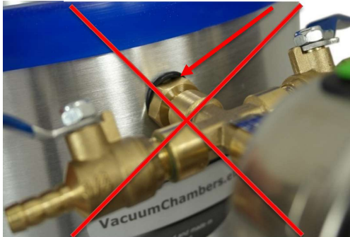
Photo 5: Incorrect position of the O-ring.
