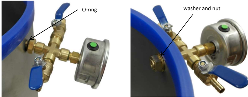
Photo 4: Air manifold inserted into the hole.
