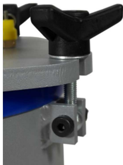
Photo 5: Correctly fastened fastener of the pressure chamber.
